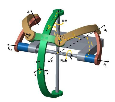
The mechanism isotropy is defined as follows; where J' are the Jacobian matrices computed numerically from the simulation data and 'm' is the order of the task space:  $\partial heta_p$  $det(\mathbf{JJ})$
