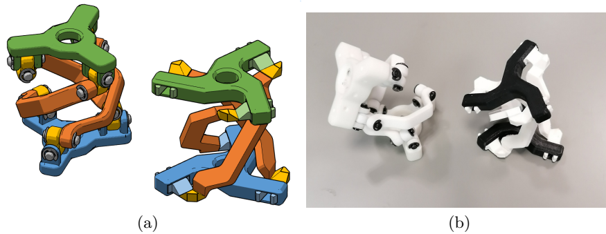
Fig. 5. Mechanism comparison. The figure presents a CAD view (a) and a photograph (b) of the two implementations of the 2DPOM mechanism considered for this work. The “traditional” design is represented on the left, while the “flexible” design on the right in both sub-figures. In (a) corresponding parts are represented with the same colours. As can be seen, the flexure-based design is considerably simpler being made with five parts instead of eleven (connection pins excluded).
